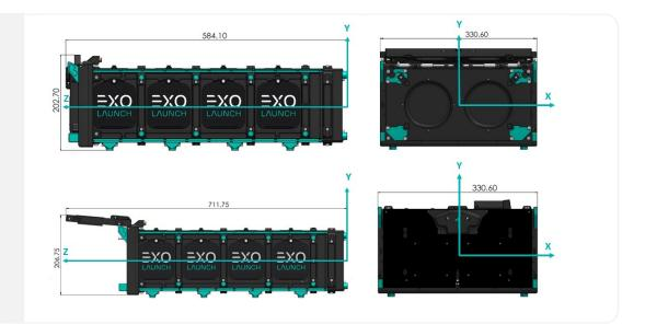
Figure 19: 12U EXOpod Nova outer dimensions.
