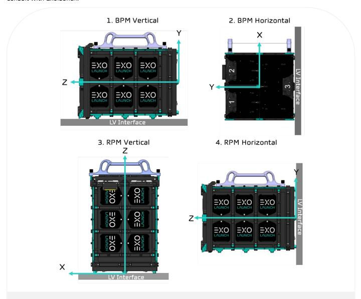
Figure 22: Rear and Bottom Plate Mounting of the EXOpod Nova in horizontal and vertical orientation.
