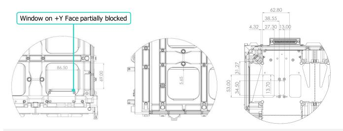
**Figure 34:** Position and dimensions of the access windows on the EXOpod Nova. The 8U is missing one row of windows whereas the 12U Nova has one fewer columns.
