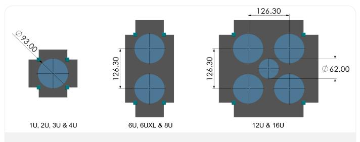
$\textbf{Figure 14:} \ \textbf{Maximum allowable tuna can dimensions for Cubesats launched in an EXOpod Nova.}$
