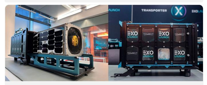
**Figure 42:** Cubesats manufactured by Kongsberg NanoAvionics being integrated into Nova and Nova TestPod using the Integration Table.
