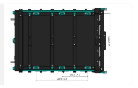
**Figure 27:** 8U and 16U Nova mounting hole pattern of the BPM interface.
