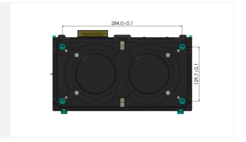
Figure 25: Mounting hole pattern of the RPM interface on the 12U and 16U Nova variants.
