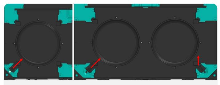
Figure 30: Clamping principle in 3U (left) and 6U (right) Cubesat slots.
