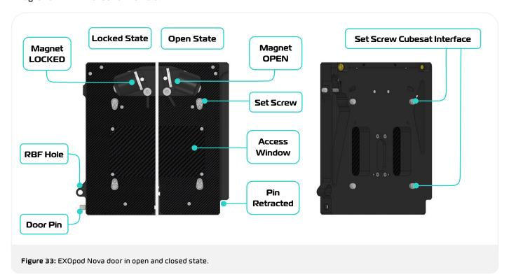
The door system is designed with a mechanism that inhibits the release of the deployment spring and wagon until the door has reached an opening angle greater than 90 deg. This system prevents the satellite from impacting the door during deployment. A latching mechanism is built into the hinge of the door, locking the door open and preventing it from rebounding once the door has fully opened.
