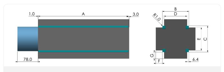
**Figure 13:** Maximum allowable dimensions for Cubesats launched in an EXOpod Nova. Contact areas with the deployer are marked in mint green.
