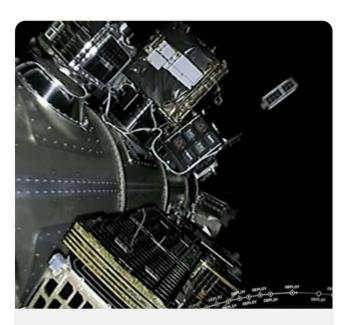
**Figure 3:** EXOpod Nova deploying a Cubesat on the SpaceX Transporter-5 mission in May 2022.
