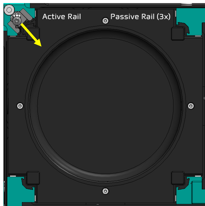
Figure 15: Clamping principle in 3U / 3U XL CubeSat slot.
