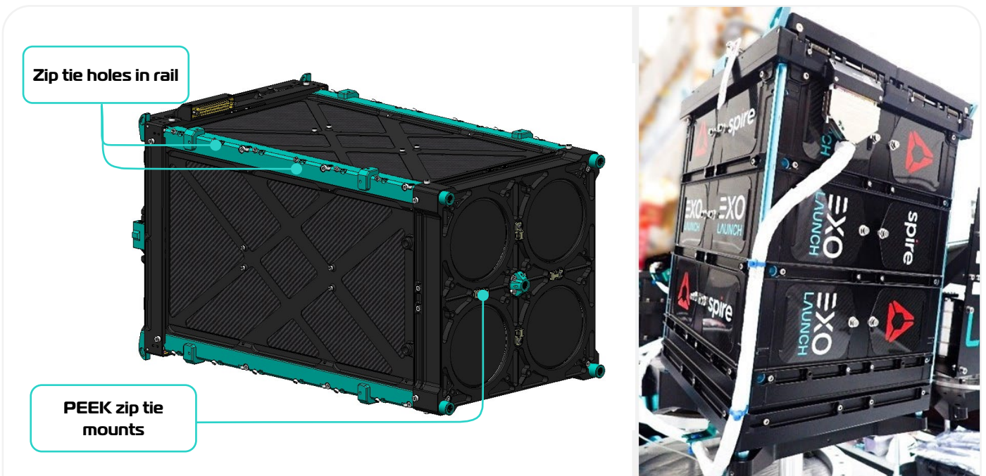
Figure 20: Left: Harness routing canal and fixation points. Right: Example of harness route.
