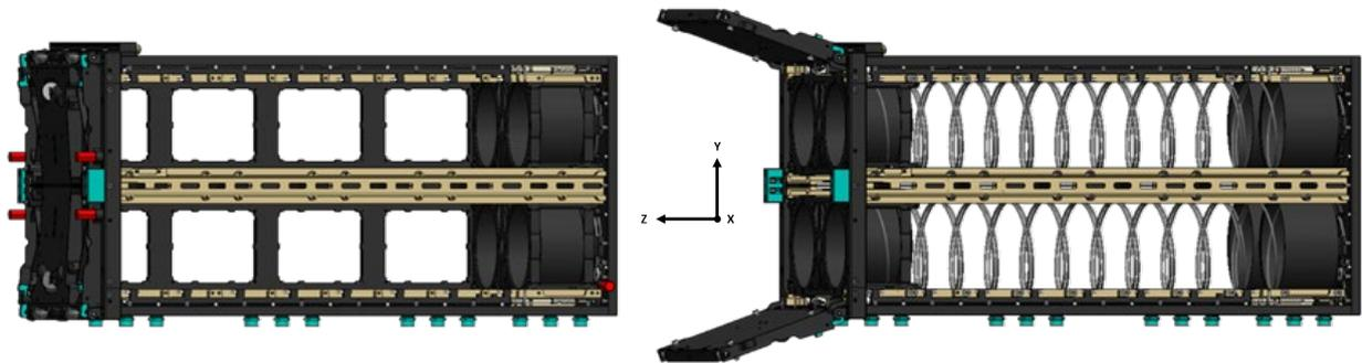
Figure 35: EXOpod 16U Bottom Plate Mounting configuration, in both closed (Left) and open (Right) states
