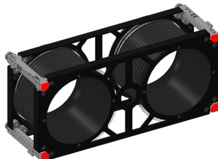
The deployment wagon is secured by its own clamping system. This mechanism will not release the spring/s until the door has opened past 90 degrees. This eliminates the possibility of the cubesat hitting the door during deployment.
