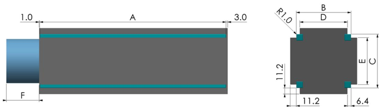
**Figure 10:** Maximum allowable outer dimensions for cubesats (3U) launched in an EXOpod Areas in contact with the deployer are highlighted in mint green
