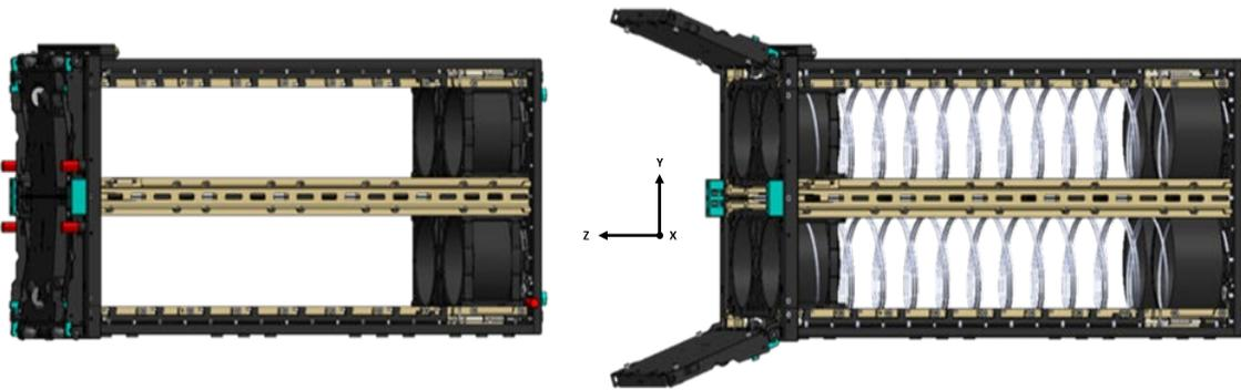
Figure 36: EXOpod 16U Rear Plate Mounting configuration, in both closed (Left) and open (Right) states
