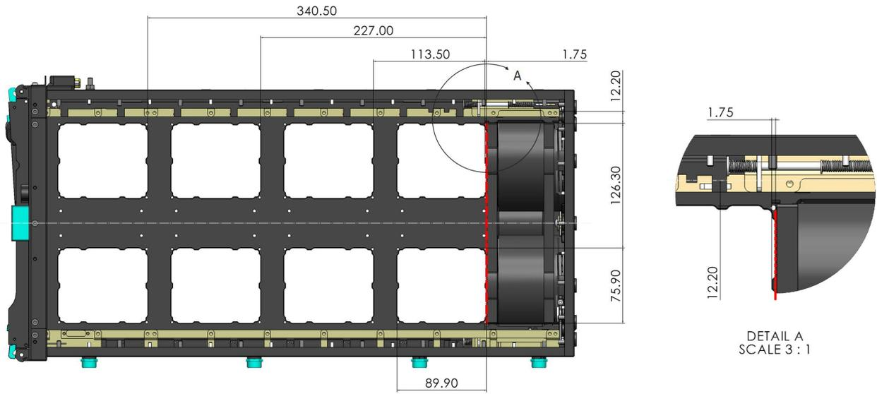
**Figure 27:** (Left) Position and Dimensions of the access windows of the 16U EXOpod. The 12U EXOpod is identical with three instead of four pairs of windows on each side. (Right) Detailed view A: Position of access window relative to the satellite contact plane
