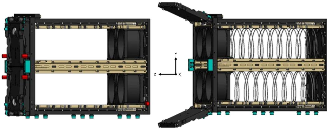
Figure 33: EXOpod 12U Bottom Plate Mounting configuration, in both closed (Left) and open (Right) states
