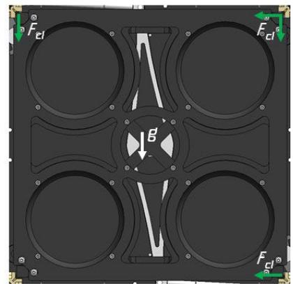
**Figure 24:** Clamping scenario based on slot size. A 3U cubesat can be clamped from any of the four corners depending on the slot it is integrated in
