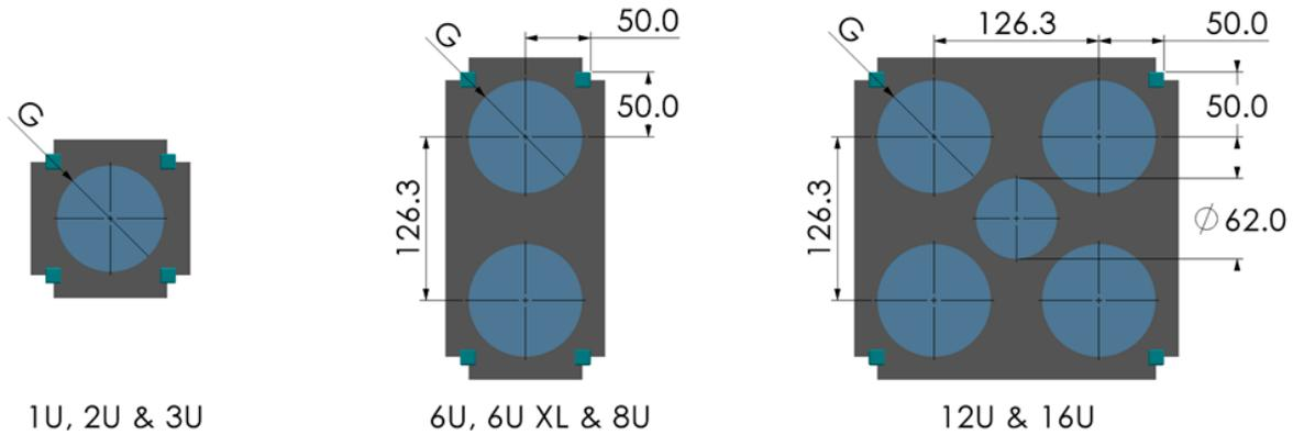
Figure 11: Maximum allowable tuna can dimensions for cubesats launched in an EXOpod
