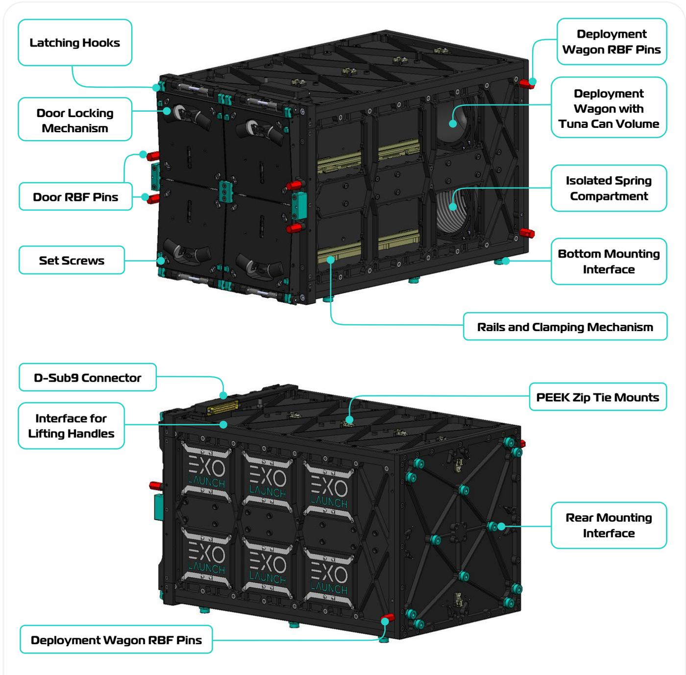
**Figure 3:** Overview of the EXOpod's main components, closed and with the deployment wagon and spring secured in the rear of the deployer
