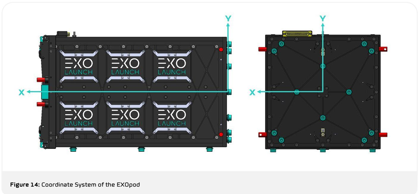
Figure 14: Coordinate System of the EXOpod
