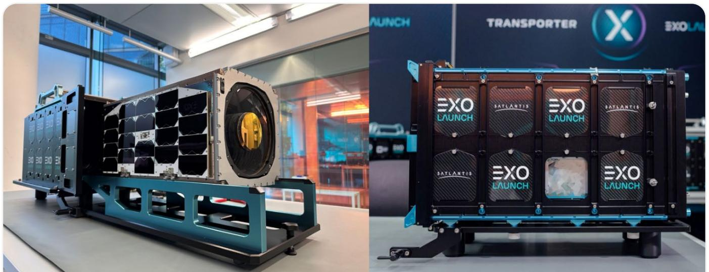
Figure 42: Cubesats manufactured by Kongsberg NanoAvionics being integrated into Nova and Nova TestPod using the Integration Table.
