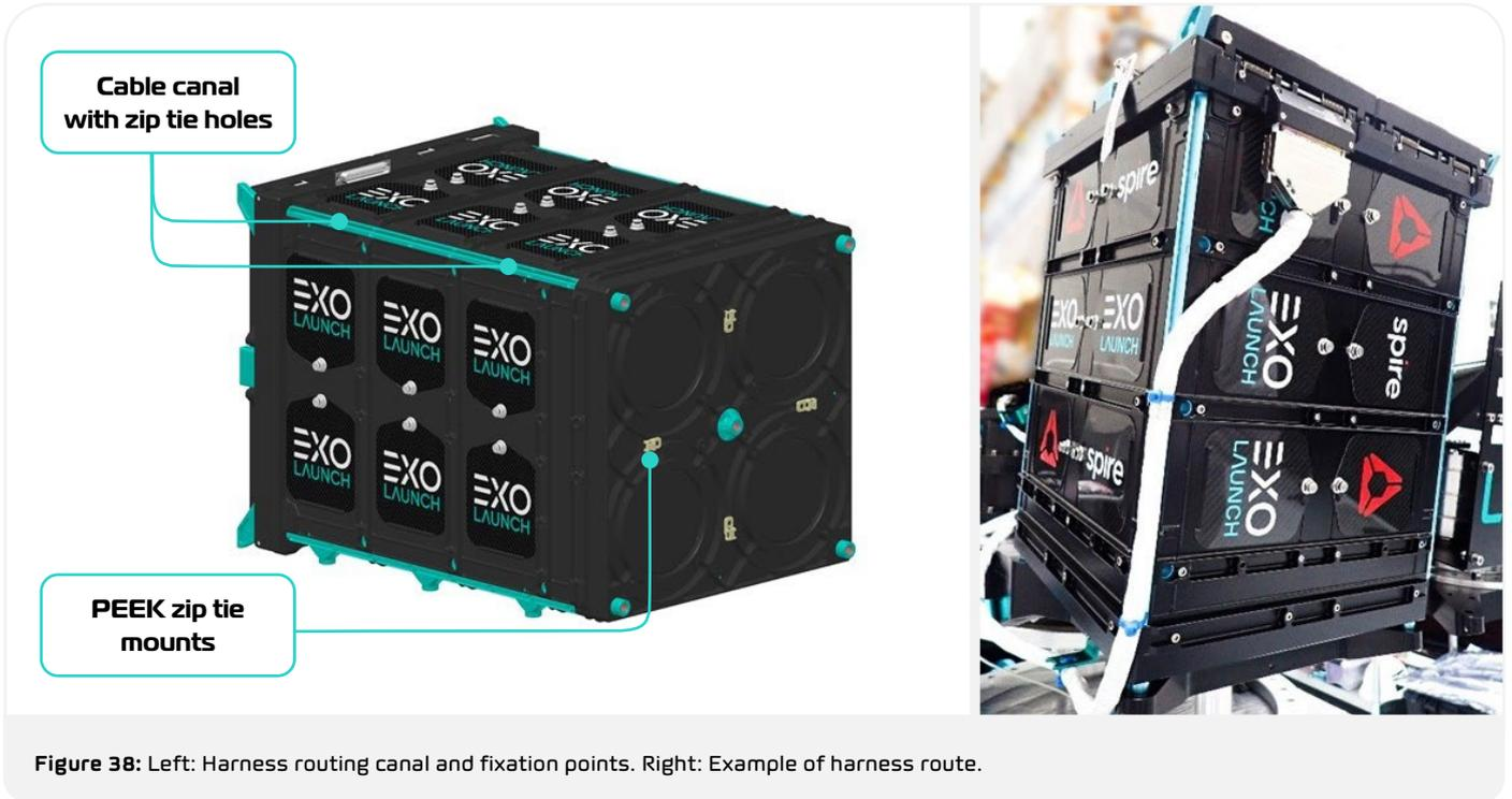
Figure 38: Left: Harness routing canal and fixation points. Right: Example of harness route.
